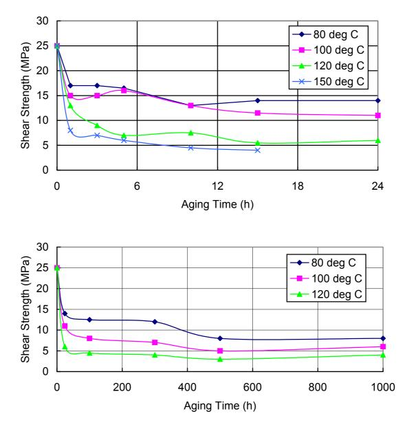
Shear Strength at Various Heating Temperatures
