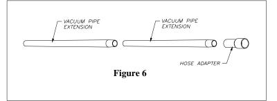
and put the other end of the 6' flexible hose into the hose adapter.
