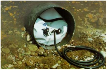
After its correct positioning into the pipeline thanks to the two handles, the stopper can be inflated with air or nitrogen through the flexible hose fitted with a valve and a safety vent valve.
