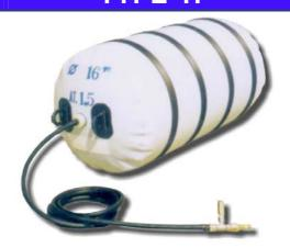
For this purpose this stopper is fitted with 4 sealing rings to improve its resistance to the residual pressure present in the pipeline. Having no metal parts, it can be abandoned inside the pipeline when friction against pipewalls breaks it. Its residual parts will be recovered at filters and pig-traps.
