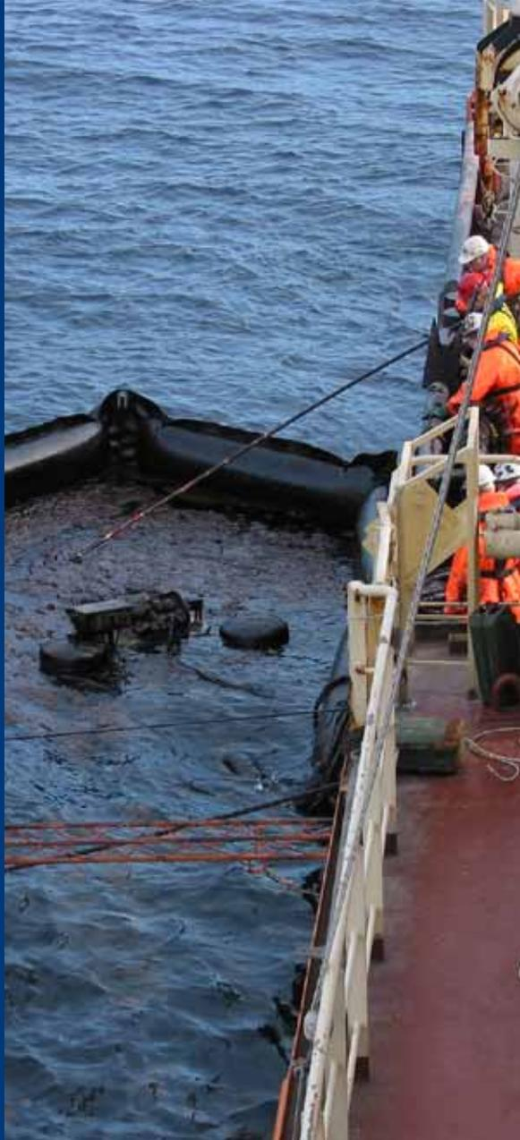
The RO-SWEEP system was originally developed for use in the harsh conditions of the North Sea to allow one vessel to conduct oil sweeping and recovery operations.
