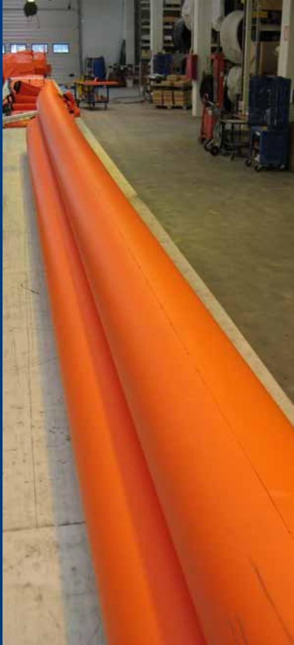
The TROILBOOM BEACH from RO-CLEAN DESMI is a lightweight versatile shore sealing boom which can be used in all situations apart from rocky shorelines.
