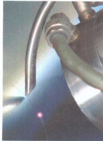
Our patented, overlap-free laser welding process allows sheets of up to 1500 mm width without leakage channels
