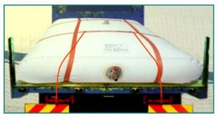
The tanks are complete of a harnessing set to fix them to the transport vehicle.
