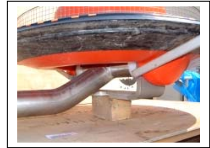
Swivel adjusts for different angles of suction hose.
