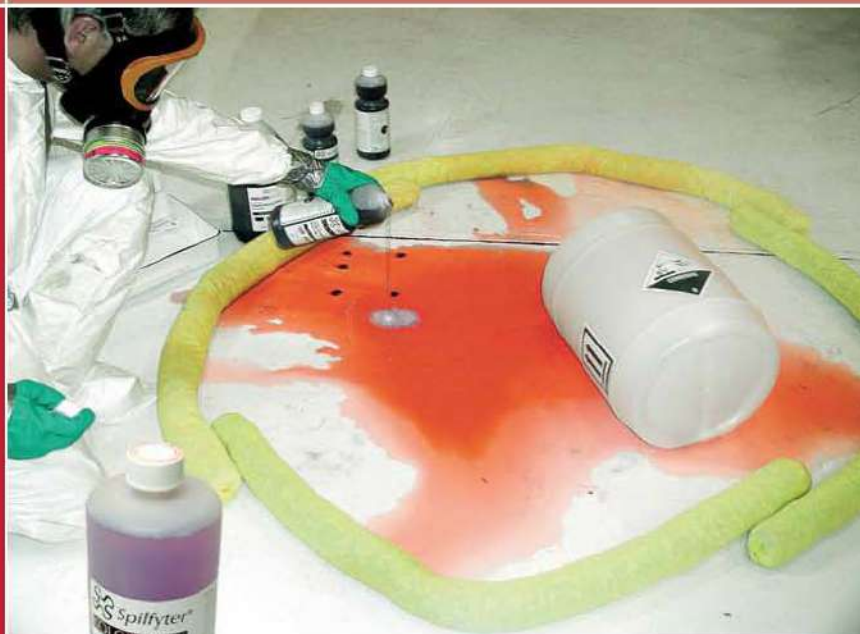
▲ Features KOLOR-SAFE® Color Change Process – Thereby Indicating When the Acid Has Been Neutralized and is Safe For Final Clean-Up.
