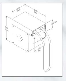
The Abanaki TubeTastic! oil skimmer can be used on machining centers with little or no access to the coolant sump from above. This unit can skim oil from chip conveyors or even totally enclosed machining centers!
