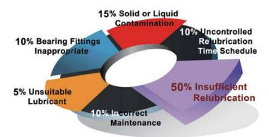
Most grease-lubricated bearings fail to reach their life expectancy. It is because that the re-lubrication procedure is unclear and/or hard to follow.
